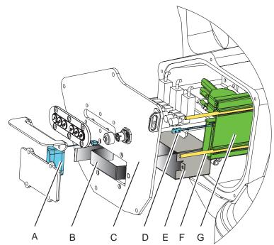
Battery pack with a 3-pole battery contact (RMU)
