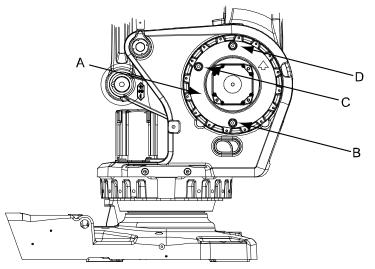
The figure shows position of gearbox, axis 3.
